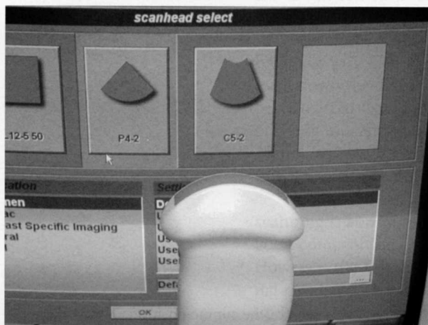
Figure 10.4. An image of a curved linear array transducer typically used for abdominal ultrasound.
