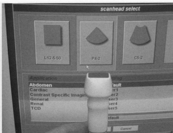
Figure 10.6. An image of a phased array transducer typically used for cardiac ultrasound but one that can be very useful for imaging the kidneys through tight rib spaces.
